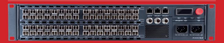
The MediorNet MetroN core router provides intense real-time signal-routing capacity (32x10G/32x4.25G ports) and offers non-blocking switching. The 2-RU device features switching delays of <40ms as well as high-speed re-routing that allows as many as 1,000 connections to be re-routed in less than a second.
