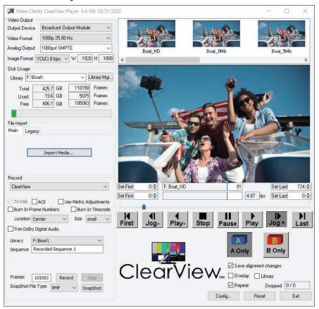
12G-SDI recording and IP capture/decoding are provided with the ClearView Player application on all systems. For playback, four 12G-SDI interfaces with one HDMI 2.0 output are included. Up to two additional video interface modules with varying capabilities may be applied as listed on page 4.
